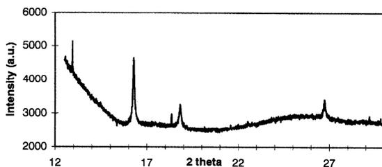
b) The presence of a second phase can be inferred from the sharp peaks observed in fig. 1 at  $12.94^\circ$  and  $18.34^\circ$ . These peaks have been indexed as the 110 and 200 peaks of a bcc structure with a lattice constant 2% larger than the fcc Pd one. Very faint 211, 220 and 310 peaks, hardly distinguishable from the noise, have been also detected.
