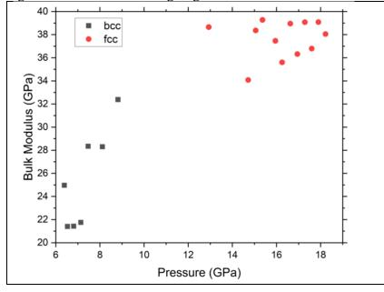
Fig 1: The pressure-dependence of the bulk modulus differ drastically between the bcc and fcc phases, with the fcc bulk modulus being almost unaffected by the pressure increase between 12-18GPa.
