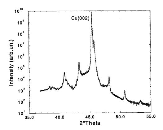
Figure 1: High-angle scan measured on Sample No. 2, showing peak (002) of the Cu(111) substrate together with the Bragg reflections corresponding to the superlattice periodicity.
