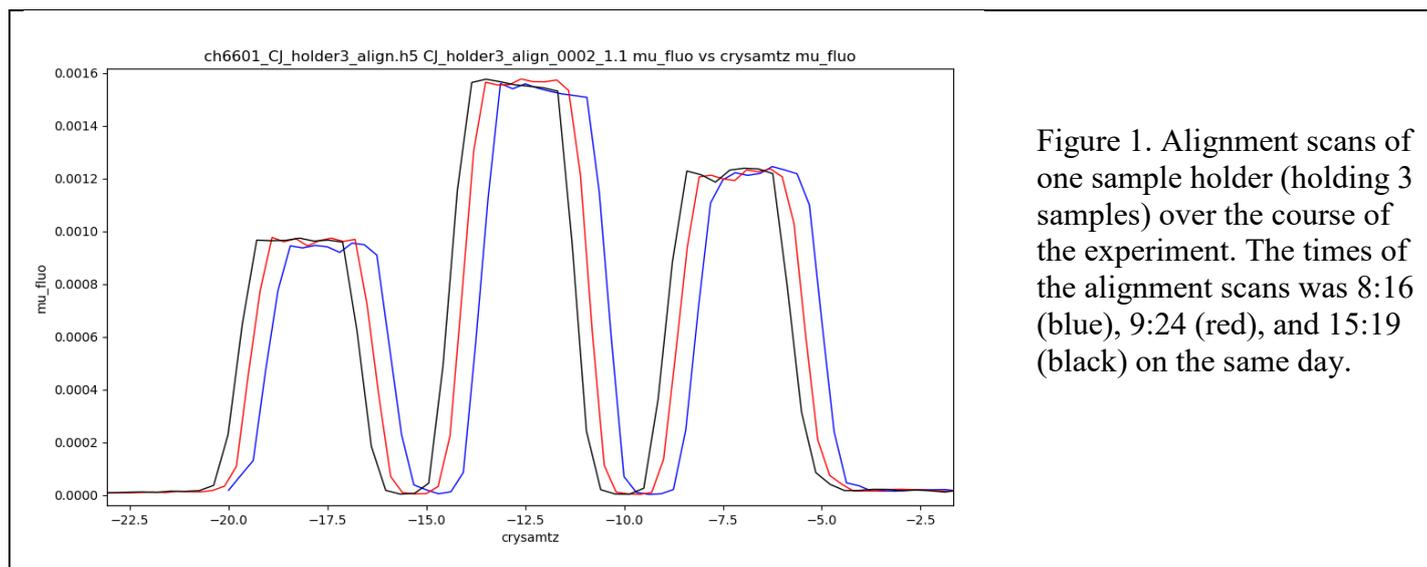
Figure 1. Alignment scans of one sample holder (holding 3 samples) over the course of the experiment. The times of the alignment scans was 8:16 (blue), 9:24 (red), and 15:19 (black) on the same day.
