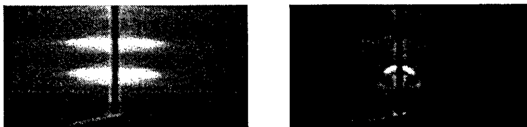
Figure 2. Non-specular X-ray reflectivity from a W/Si multilayer grating. Measurement at two different azimuths: 0^\circ (perpendicular to wires, left) and 90^\circ (parallel to wires, right). The RDS-sheets are inclined. The discussed bright arc of many coherently excited grating truncation rods is visible in the figure on the right.
