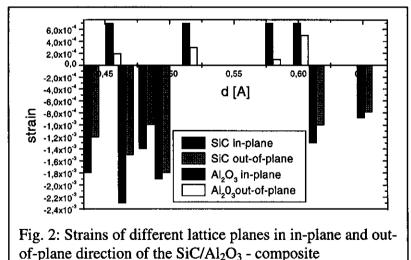
The value of theses strains due to elastic ansiotropy is slightly different for different lattice planes.
