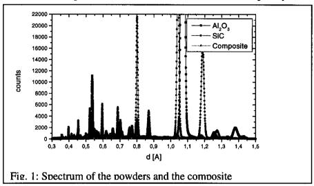
The spectra indicate that strong peak overlapping is present. The position of the reflections in spectra recorded at different times proved to be higly reproducible (difference between 5 E-5 nm typically). The strain obtained in in-plane and out-of-plane direction in good agreement with neutron diffraction revealed compressive residual strains in the SiC and tensile residual strains in the  $Al_2O_3$  (fig.2).
