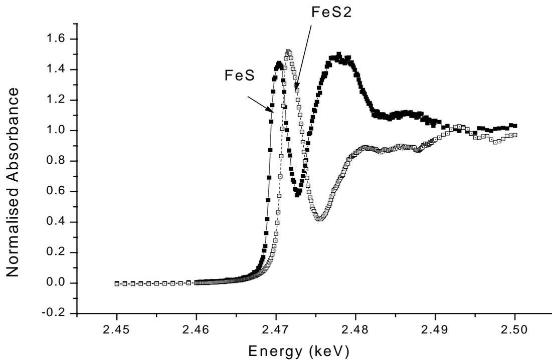
Figure 2: XANES spectra of FeS and FeS<sub>2</sub> in the same experimental conditions
