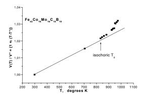
Left: Isentropic  $T_g$  determined calorimetry Right: Isochoric  $T_g$  determined from diffraction data Recent joint publications with the participation of the ESRF:
