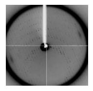
At the moment, we are trying to improve conditions for cryoprotection of these crystals in order to extend the resolution limit and to decrease radiation damage.
