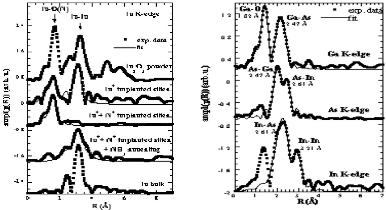
Fig. 1,2. Moduli of Fourier transforms (experimental data and fits) for the samples doped with In together with standard of In bulk and  $\text{In}_2\text{O}_3$  powder (left) and for the triple-implanted sample at the respective three edges (right).
