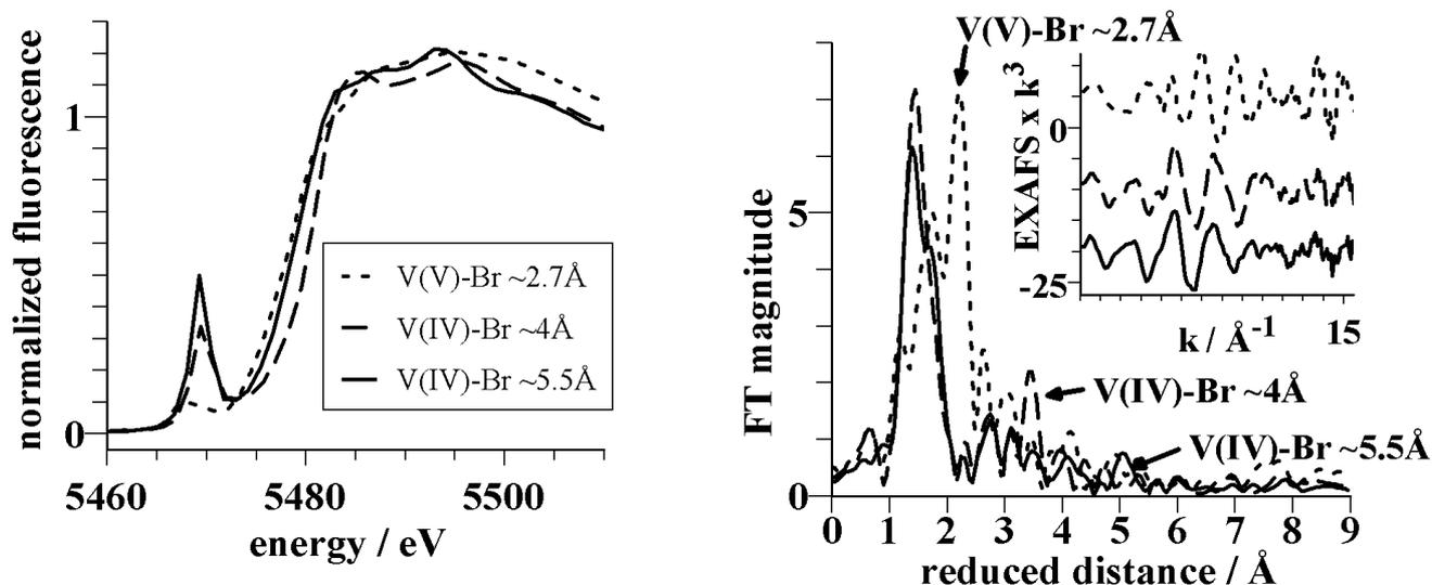
**Fig. 1:** (A) XANES spectra at the V K-edge for three selected synthetic vanadium model compounds with different V-Br distances. (B) EXAFS spectra of the models in (A). Fts calculated for energies ranging from 20 eV to 950 eV above  $E_0$ .
