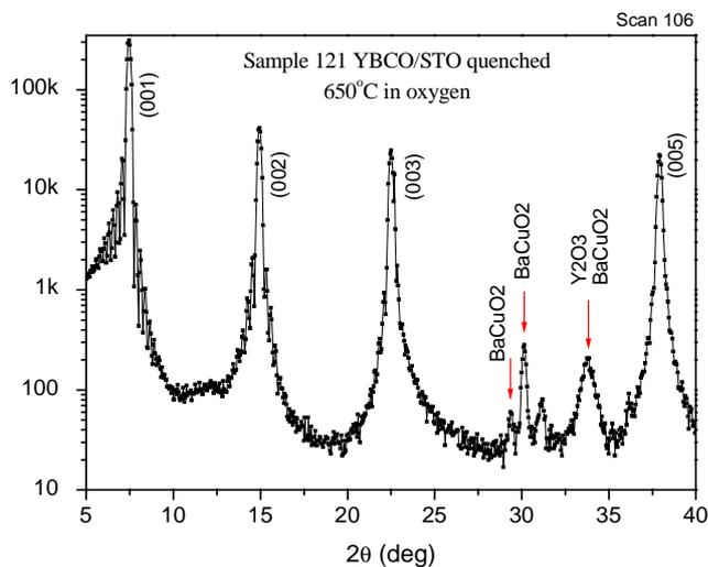
**Fig. 4:** YBCO/STO scan at the beginning of the oxygen uptake. Scan at 650°C.
