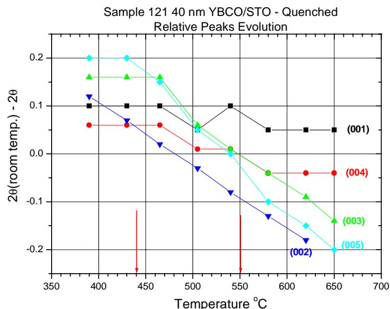
**Fig. 2:** The relative peaks evolution for 40 nm quenched YBCO/STO.
