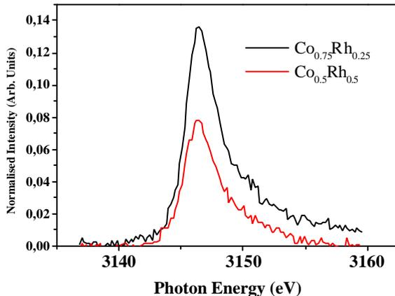
**Fig. 3 :** XMCD signals at  $L_2$  edges for Coll. 1 and Coll. 2.  $\mu_0H = 7$  T,  $T < 10$  K
