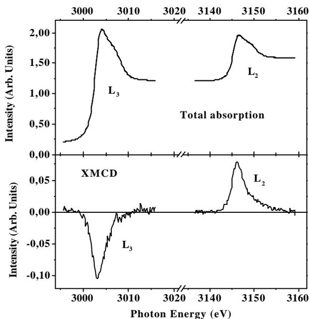
**Fig. 1** : total absorption and XMCD signals at  $L_3$  and  $L_2$  edges of Coll. 1.  $\mu_0H = 7 \text{ T}$
