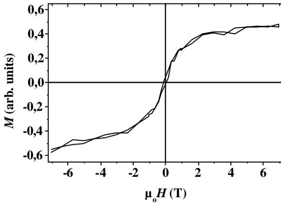
**Fig. 2 :** Magnetization loop of Coll.1 measured at the  $L_2$  threshold (3.146 keV).  $T < 10$  K
