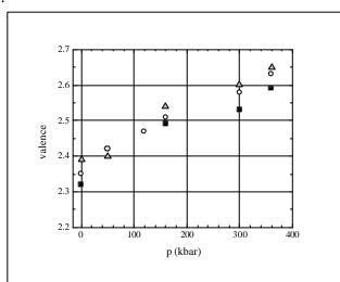
Fig. 4. Valence values estimates from the analysis of  $La_I$  Partial Fluorescence Yield (circles) and  $L_3$  Resonant Inelastic X-Ray Emission spectra (vs.  $h\mathbf{n}_{IN}$  with triangles, well below threshold with squares).
