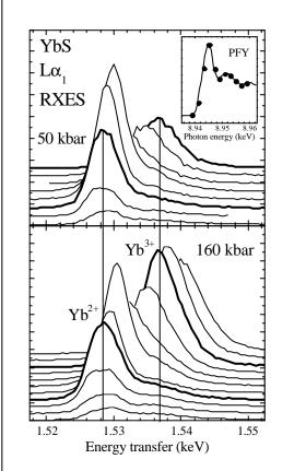
Fig. 2. RXES spectra of YbS at selected energies indicated in the inset.
