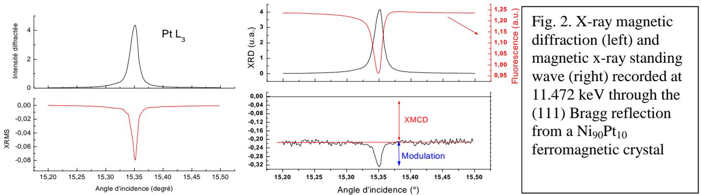
Fig. 2. X-ray magnetic diffraction (left) and magnetic x-ray standing wave (right) recorded at 11.472 keV through the (111) Bragg reflection from a Ni<sub>90</sub>Pt<sub>10</sub> ferromagnetic crystal
