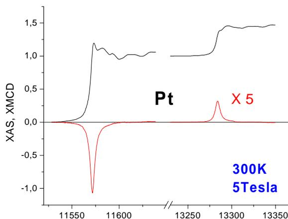
Fig. 1. XAS and XMCD spectra from the Ni<sub>90</sub>Pt<sub>10</sub> crystal at the Pt L<sub>2,3</sub> edges.
