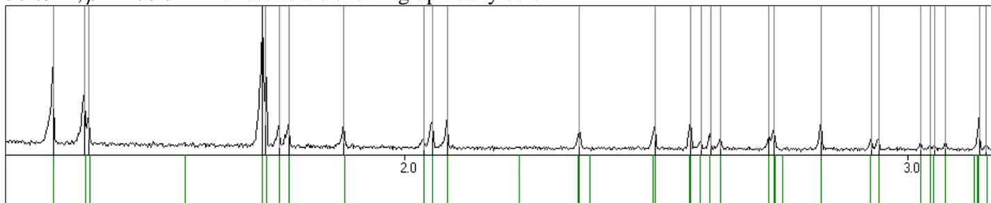
These unit-cell values are in good agreement with single-crystal crystallographic studies of this enzyme in this particular crystal form. The indexing revealed one problem: the peaks were so sharp that our default bin size of  $0.001^\circ$  proved too large, and rebinning was required.
