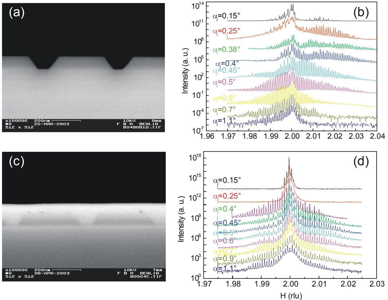
**Figure 2:** SEM pictures of the of freestanding (a) and overgrown (c) gratings using the optimized stressor layer sequence; the corresponding X-ray pattern are shown in (b) and (d), respectively.
