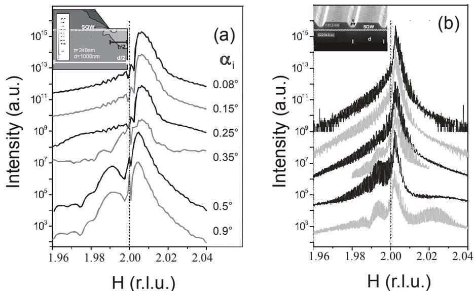
**Figure 1:** Simulated (a) and experimental (b) GID X-ray pattern (longitudinal scans) for different penetration depths for the sample as a shown in the inset (inset (a): model; inset (b) real structure).
