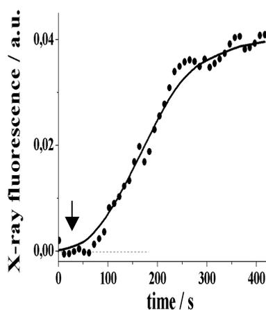
**Figure 2:** Timescan of X-ray fluorescence at 4038 eV. Arrow: duration of EXAFS scans.
