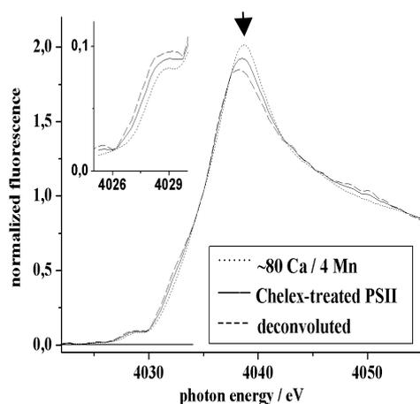
**Figure 1:** Ca XANES spectra of PSII samples. Dashed line: tentative pure spectrum of the Ca bound to the Mn complex obtained by deconvolution. Inset: pre-edge peak region.
