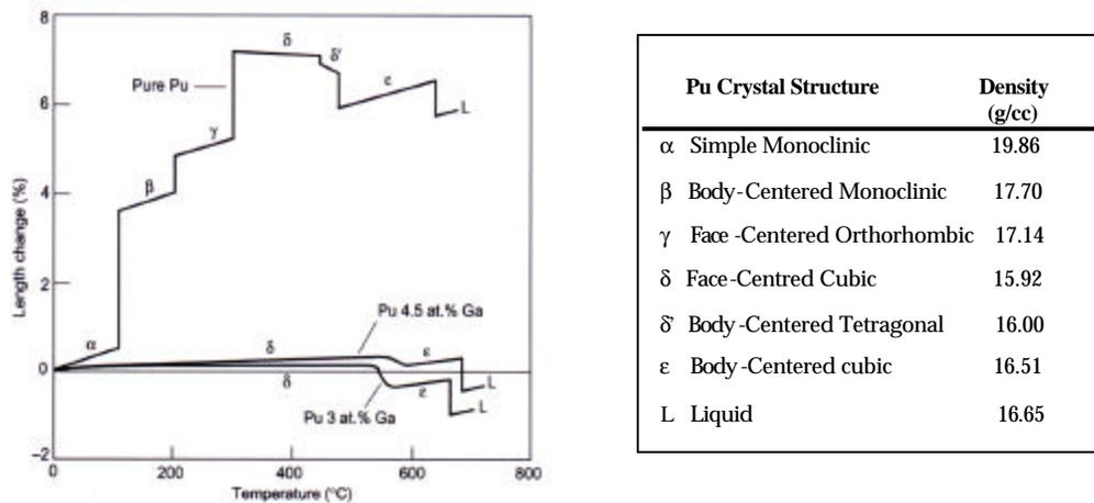
**Figure 1** Transformations in Pu to different crystal structures are accompanied by very large volume changes. Alloying with Ga or Al avoids the transformation to  $\gamma$ ,  $\beta$  and  $\alpha$  and stabilizes the  $\delta$  phase all the way to room temperature and below [1].
