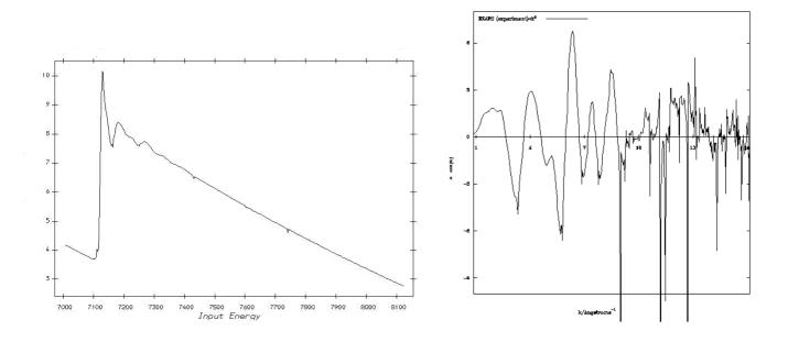
Figure 1: The Fe K-edge absorption spectrum (left) and its  $k^3$  weighted EXAFS spectrum (right) of an iron and cobalt-containing spinel.
