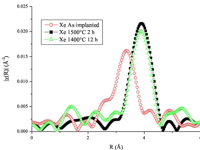
Figure 2 : Fourier transforms of the Xe K edge EXAFS spectra.
