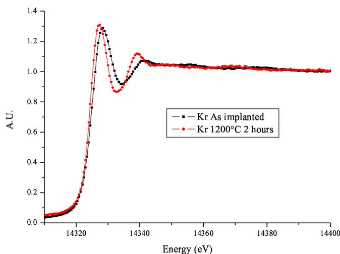
Figure 1 : XANES spectra obtained at the Kr K edge.
