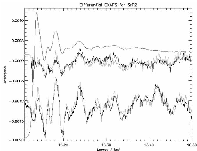
Fig 5: Differential EXAFS for powdered  $\text{SrF}_2$ . The top set is for  $\Delta T = 1.4 \pm 0.2 \text{K}$ , and the lower set for  $\Delta T = 2.8 \pm 0.2 \text{K}$ . The original EXAFS is at the very top. Gas flow was set to 5lpm. The grey lines are the gas jet phase shifted signals inverted.
