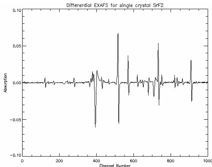
Fig 4: Differential EXAFS for single crystal  $\text{SrF}_2$ . The expected signal has been destroyed by Borrmann transmission glitches. Compare with Fig 5.
