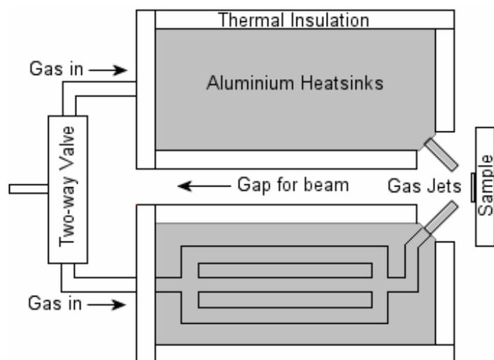
Fig 1: A Schematic representation of the gas jet apparatus
