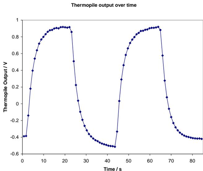
Fig 3: A typical thermopile response signal. Gas flow was set to 4lpm, and  $\Delta T = 2.8 \pm 0.2 \text{K}$ . Gas valve was switched every 20s
