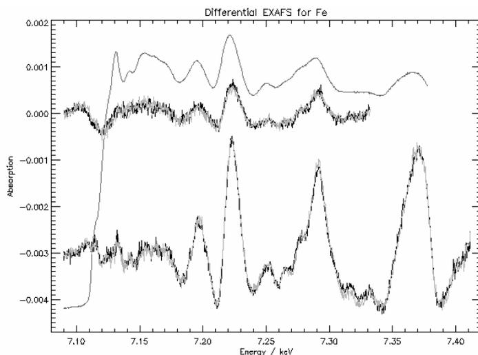
Fig 6: Differential EXAFS for polycrystalline Fe. The top set is for  $\Delta T = 1.4 \pm 0.2 \text{K}$ , and the lower set for  $\Delta T = 2.8 \pm 0.2 \text{K}$ . Gas flow was set to 5lpm. The grey lines are the gas jet phase shifted signals inverted.
