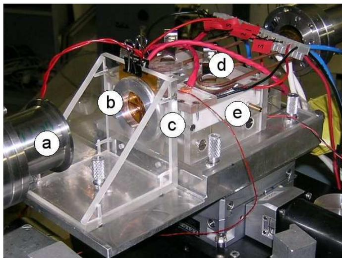
Fig 2: The actual gas jet mounted in the beam. a) beam in, b) thermopile with sample, c) gas jets behind here, d) heaters and sensors, e) heatsink.
