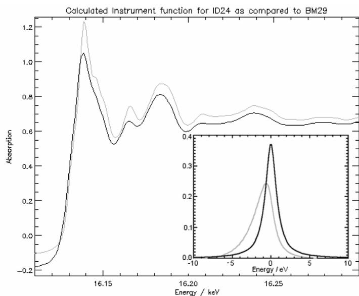
Fig 7: Instrument function corrections to match BM29 data to that from ID24. The black line in main graph shows the calculated absorption spectrum of ID24 resulting from convolutions to the corresponding BM29 spectrum (grey). The insert shows the convolution function (grey line), which results from combining a lorentzian of width  $3.4 \text{eV}$  (black line) with a function that is zero in  $-\infty \leq E \leq 0$  and an exponential decay of width  $1.2 \text{eV}$  in  $0 < E \leq \infty$ .
