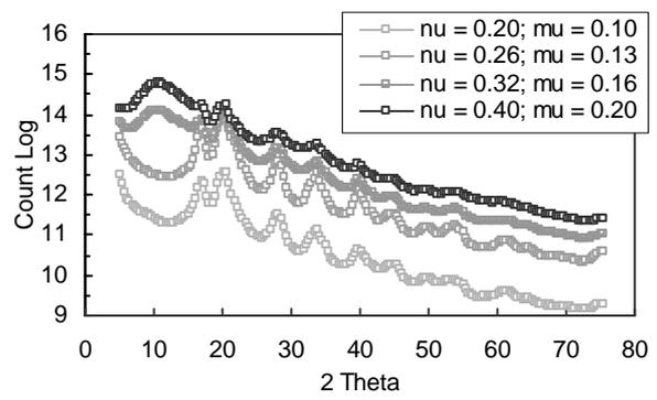
Figure 4: Diffraction spectra for cobalt clusters deposited on glass.
