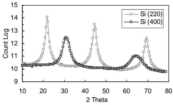
Figure 1: Bare silicon substrate along the (220) and (400) directions.
