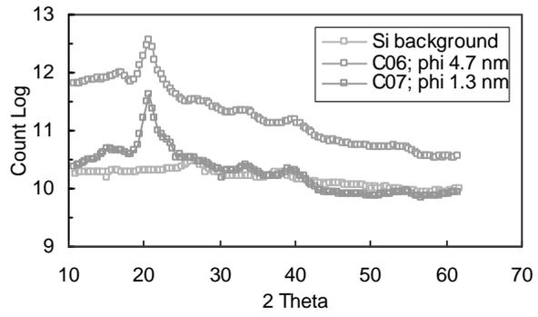
Figure 2: Cobalt clusters diffraction spectra obtained by data clipping from two Si direction scans.
