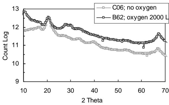
Figure 3: Diffraction spectra for oxidized (B62) and un-oxidized (C06) clusters.
