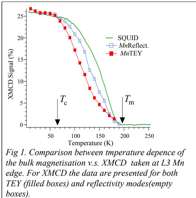
Fig 1. Comparison between temperature dependence of the bulk magnetisation v.s. XMCD taken at L3 Mn edge. For XMCD the data are presented for both TEY (filled boxes) and reflectivity modes (empty boxes).
