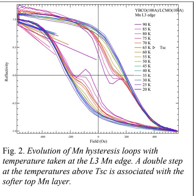
Fig. 2. Evolution of Mn hysteresis loops with temperature taken at the L3 Mn edge. A double step at the temperatures above  $T_{sc}$  is associated with the softer top Mn layer.
