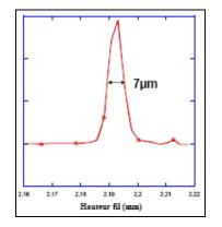
**Figure 1** (left): spot size defined as the FWHM of the fluorescence signal given by scanning a Cu wire (
