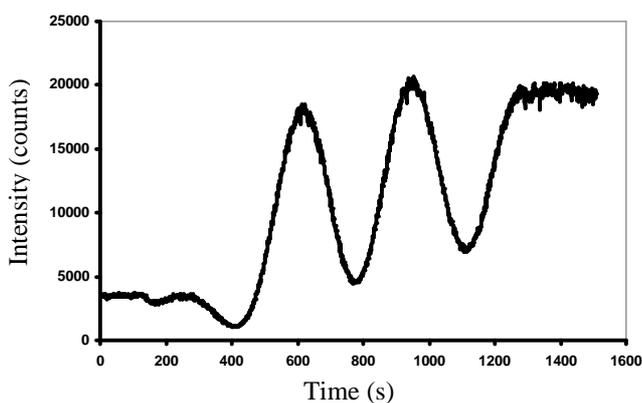
Fig. 1: The intensity of the reciprocal point (0,0,0.5) during 1 deposition of  $\text{PbTiO}_3$  on  $\text{SrTiO}_3$  at  $500^\circ\text{C}$ . After starting the laser for deposition, due to roughening the intensity decreases, and finally upon completion of the layer the surface is smooth again, hence a maximum.
