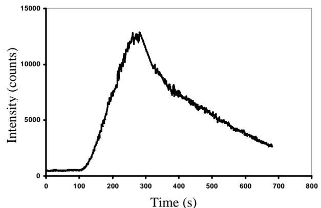
Fig.2: The intensity of the reciprocal point (0,0,0.5) during deposition. After starting the laser, the intensity increases but after the laser is turned off (270 sec.) the intensity drops because the layer is unstable.
