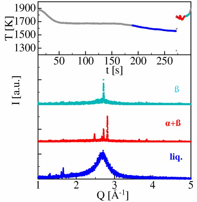
**Figure 2:** Energy dispersive X-ray diffractograms acquired during an undercooling experiment on a  $\text{Ti}_{40}\text{Al}_{50}\text{Nb}_{10}$  melt. The temperature-time profile is shown in the upper part of the figure. The different colours mark the time intervals during which the diffractograms plotted in the same colour were recorded.
