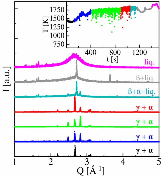
**Figure 1:** Energy dispersive X-ray diffractograms acquired during slow heating of a  $\text{Ti}_{40}\text{Al}_{50}\text{Nb}_{10}$  sample. The temperature-time profile of this experiment is shown in the insert. The different colours mark the time intervals during which the diffractograms plotted in the same colour were recorded.
