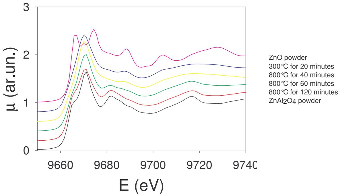
**Figure 2:** Zn K-edge XANES spectra of ZnO onto  $\text{Al}_2\text{O}_3$  (0001) single crystal after different treatments. For comparison purposes the inset also shows the spectra of ZnO and  $\text{ZnAl}_2\text{O}_4$  powders.
