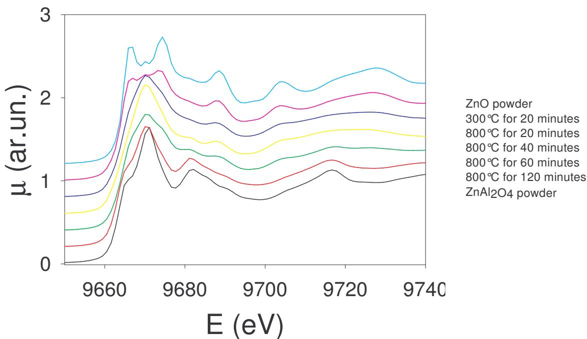
**Figure 1:** Zn K-edge XANES spectra of ZnO onto  $\text{Al}_2\text{O}_3$  (11-20) single crystal after different treatments. For comparison purposes the inset also shows the spectra of ZnO and  $\text{ZnAl}_2\text{O}_4$  powders.
