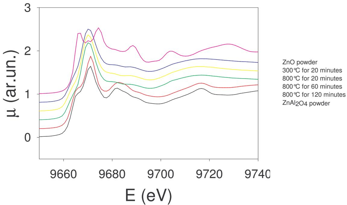
**Figure 3:** Zn K-edge XANES spectra of ZnO onto  $\text{Al}_2\text{O}_3$  (0001) single crystal after different treatments. For comparison purposes the inset also shows the spectra of ZnO and  $\text{ZnAl}_2\text{O}_4$  powders.
