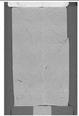
Figure1: vertical slice through tomography image of LBU1 Beaucaire marl sample at the end of the test
