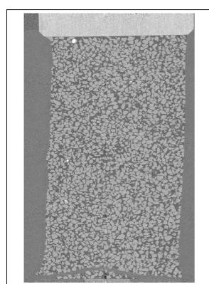
Figure 2: Vertical slice through the tomography image of the S28\_SYN2 Hostun Sand sample at the peak load
