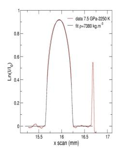
Fig.1: Absorption scan in liquid Fe at 7.5 GPa (the peak on the right hand side of the scan corresponds to the Pt foil inserted for P-T calibration purposes).
