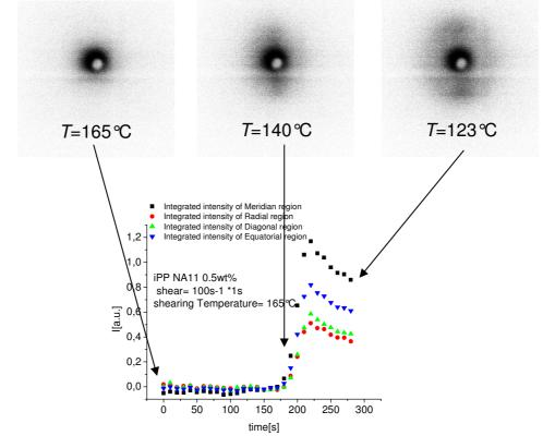
**Figure1**.2DSAXS images and integrated intensity of iPP-NA11 0.5wt% as a function of time after applying a shear of 100 ( $100s^1$  for 1 s) at *T*=165°C.
