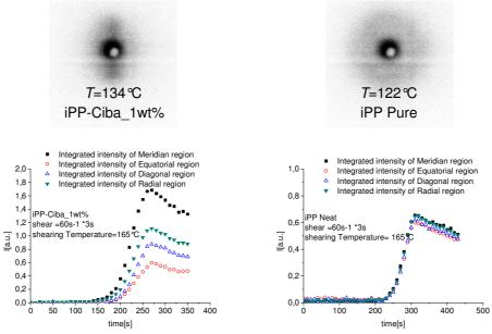
**Figure3**.2DSAXS images and integrated intensity of iPP-Ciba 1wt% and pure iPP as a function of time after applying a shear of 60 ( $60s^{-1}$  for 3 s) at *T*=165°C.
