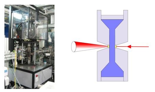
The experiments performed concern the study of the early stages in the flow induced crystallization of polymers, mainly isotactic polypropylene, iPP. The results obtained during this experiment highlight the formation of an highly oriented 'shear layer' when the applied stress overcomes a certain threshold that depends on the material, on its molecular weight and on the experimental temperature.
