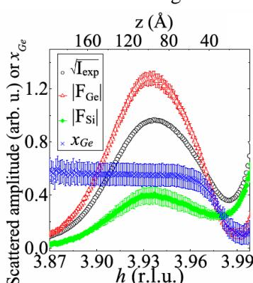
the scattered intensity ( $\sqrt{I_{\text{exp}}}$ ) close to the in-plane Si(400) Bragg reflection, the modulus of the Ge and Si structure factors, as well as the Ge content, as a function of reciprocal unit  $h$  and island height  $z$ . Considering the Ge concentration for  $h$  lower than 3.97, the results clearly show a strong intermixing phenomenon leading to an island composition of about 60% Ge together with a slight linear increase of Ge concentration below  $h = 3.97$ .
