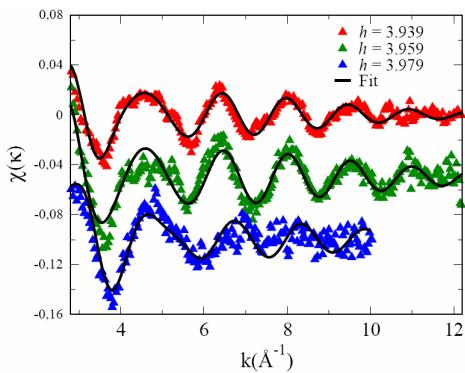
Figure 2. Raw EDAFS spectra (triangles) and best fit curves (solid lines) recorded at three different  $h$  values (3.939, 3.959 and 3.979) from top to bottom. Curves are shifted for sake of clarity.
