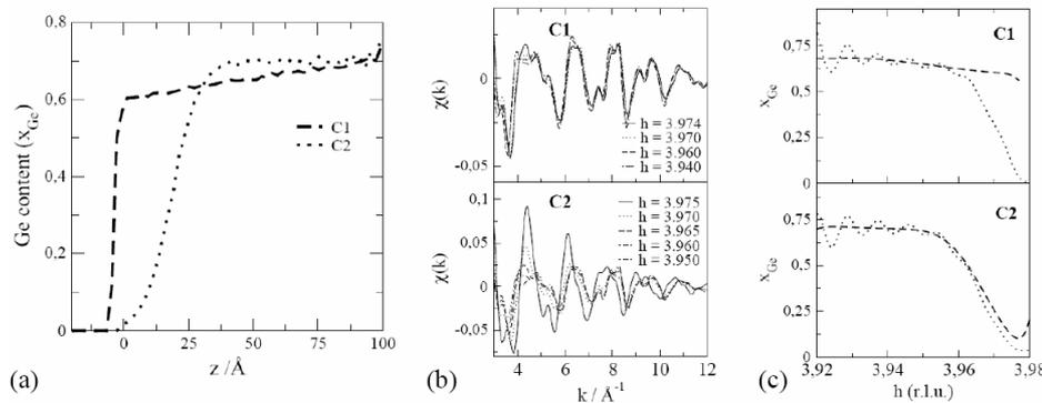
Fig. 3 (a) Chemical composition profiles for GeSi/Si(100) island models C1 and C2. (b) Extended DAFS calculated as a function of reciprocal unit  $h$  for models C1 and C2. (c) Ge concentration extracted back from the simulated MAD of models C1 and C2.
