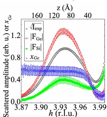
Figure 1.  $\sqrt{I_{\text{exp}}}$  measured at 11.053keV (50eV below Ge K-edge) and at an incident angle  $\alpha_i = 0.1^\circ$ ,  $|F_{\text{Ge}}|$ ,  $|F_{\text{Si}}|$  and Ge composition  $x_{\text{Ge}}$  plotted as a function of  $h$  around Si(400) and as a function of island height  $z$ .
