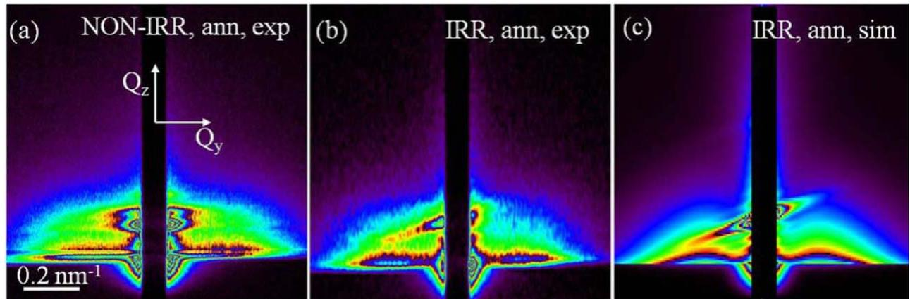
Fig. 1 Measured (a,b) and simulated (c) GISAXS intensity maps of a non-irradiated (a) and irradiated (b,c) Ge+SiO<sub>2</sub>/ SiO<sub>2</sub> multilayer.
