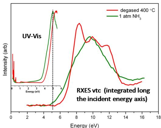
Figure 2. Comparison between UV-Vis spectra (left) and RXES (right - with incident energy integrated).
