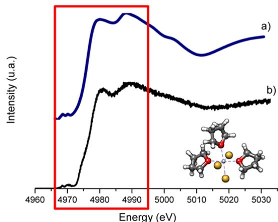
Figure 3. XANES spectra for  $\text{Ti}(\text{THF})_3\text{Cl}_3$ . (bottom) Experimental vs (top) calculated spectra by means of FDMNES.
