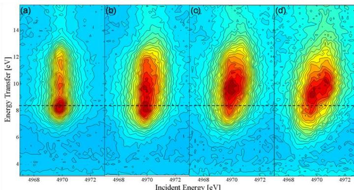
Figure 1. vtc RXES maps for (a) TS-1 degassed (b) in presence of H<sub>2</sub>O in liquid phase (c) in presence of 1 atm of NH<sub>3</sub> (d) in presence of H<sub>2</sub>O/H<sub>2</sub>O<sub>2</sub> solution
