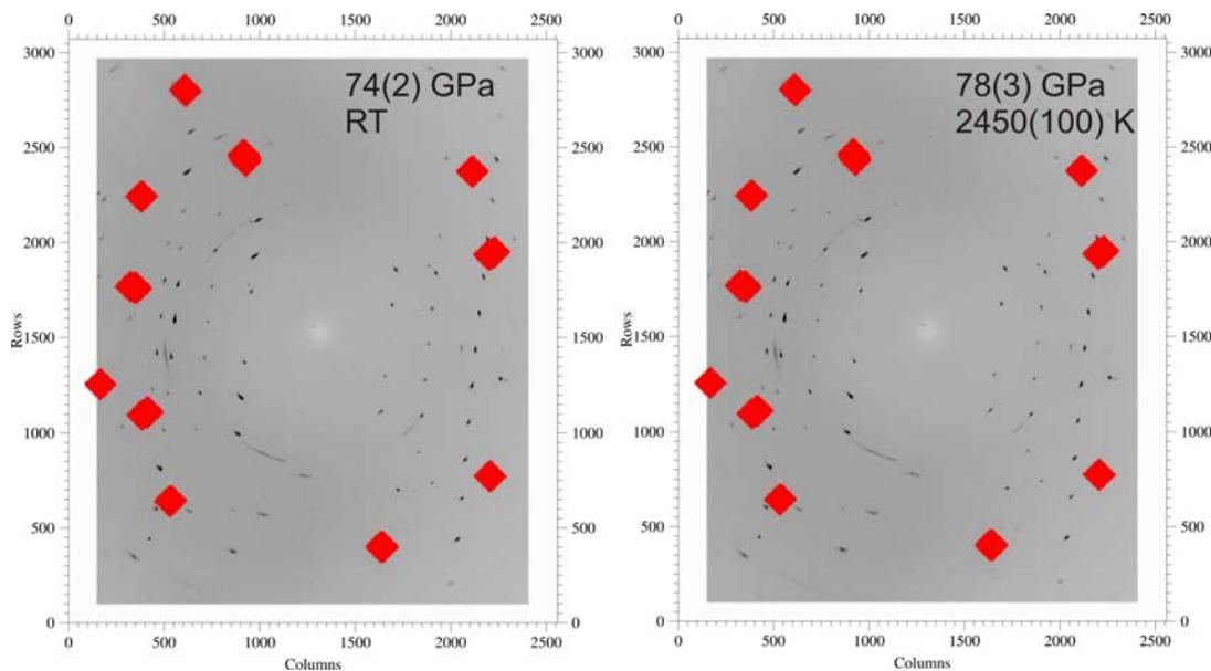
Fig. 2. Example of rotational (40 degree) X-ray diffraction images of silicate perovskite compressed in Ne pressure medium (arcs) collected before (left) and during (right) laser-heating in DAC (diamond peaks are masked).
