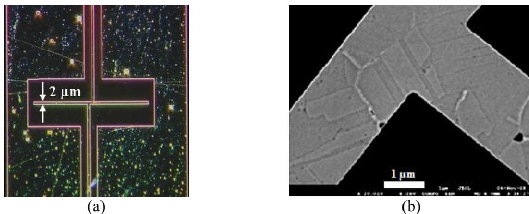
Figure 1- X-ray fluorescence cartography to locate the copper lines (a). SEM observation of the microstructure of a Cu-MEMS sensor showing small twinned grains (b).
