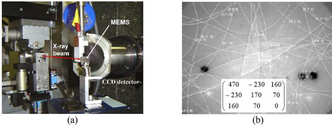
Figure 2- Experimental setup to acquire Kossel line patterns in ID13 beamline (a). A Kossel line pattern obtained for a copper grain located at the extremity of the pointer, with the simulated pattern superimposed and the full stress tensor result (in MPa) (b).
