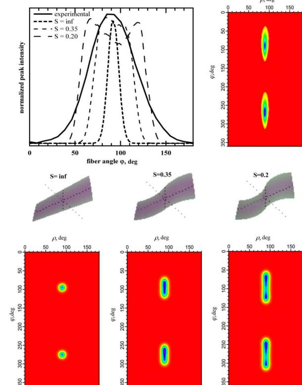
Figure 3. Comparison of the simulated and experimental peak broadening. (Top left) The fiber-angle profile of the equatorial 010 reflection for the experiment (solid) and simulation (dashed). (Top right) Experimental 2D-profile of the 010 reflection. (Middle row) Cartoons of the lamellae with different S-shape parameter indicated above the diagrams and the corresponding 2D plots (bottom row) of the simulated 010 reflection intensity.
