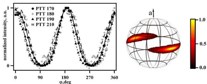
Figure 2. Normalized integral intensity of the 010 reflection as a function of the fiber angle  $\phi$  for different crystallization temperatures of PTT indicated on the graph (left). The curves reveal virtually no variation of the fiber-angle broadening with crystallization temperature. Pole figure corresponding to the 010 reflection (right).
