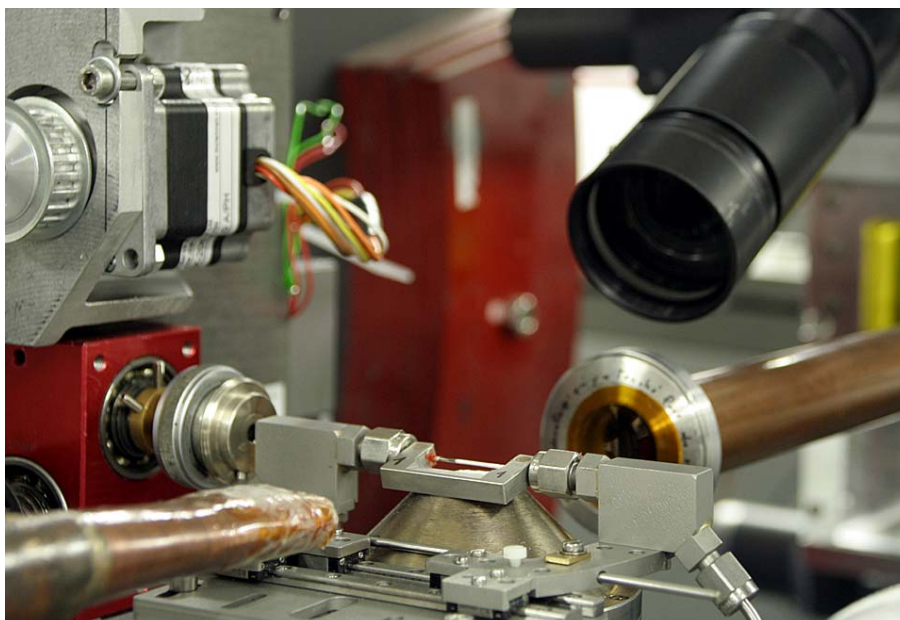
Figure 1: Reactor set-up for in situ XAS/XRD/Raman measurements
