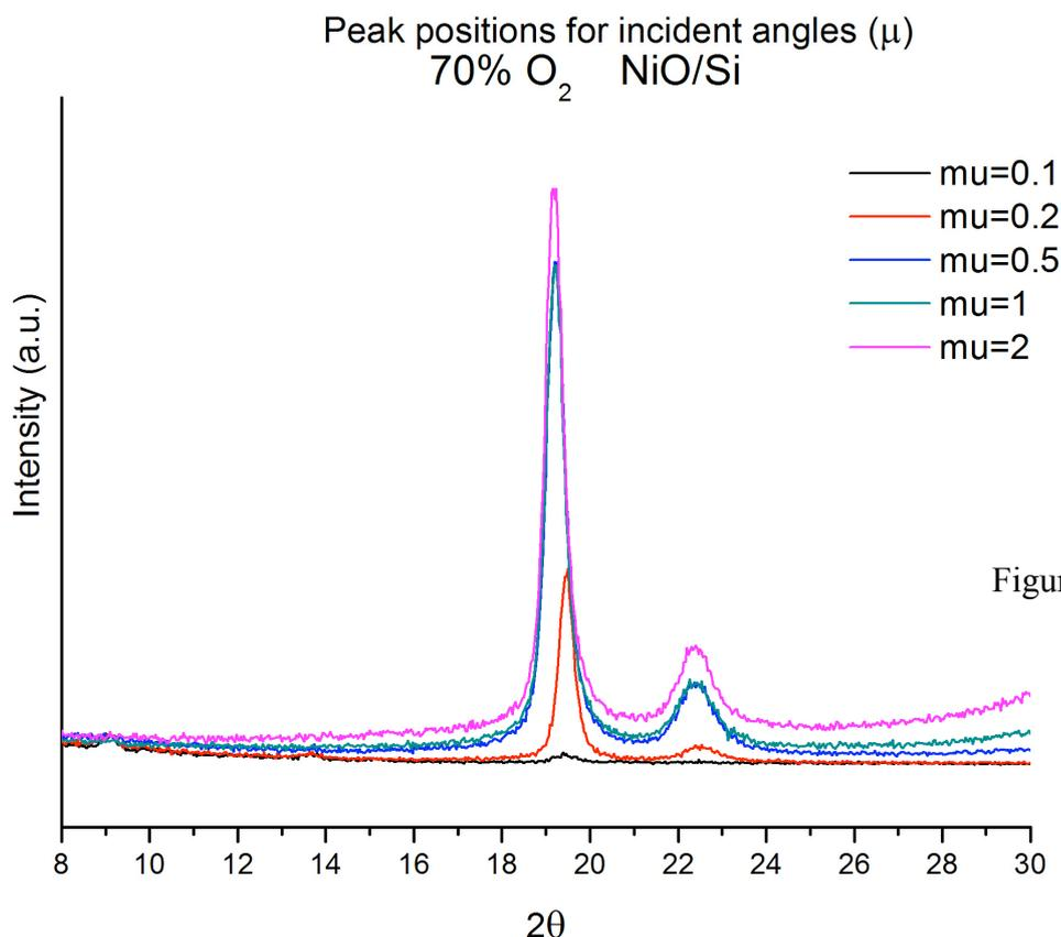
Figure 1 the diffraction pattern, obtained for the sample grown with 70% oxygen in the plasma, on a silicon substrate. There is a clear shift of the (111) peak towards higher angles as the incidence angle decreases, suggesting a change in the lattice constant as with depth: the lattice parameter would be higher closer to the interface.
