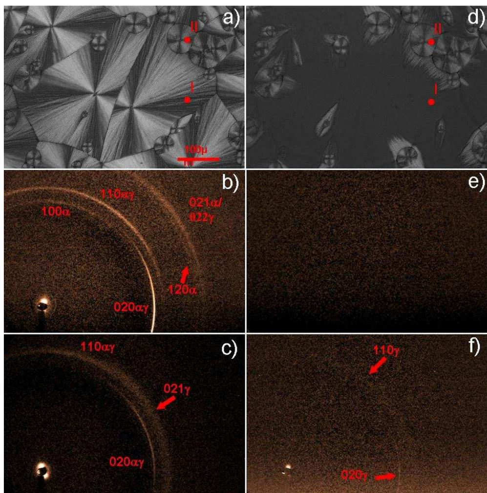
Figure 1. Structural characteristics of the PVDF film at room temperature (left column) and 180°C (right column). Optical microscopy images (A,D), the red circles indicate the measurements points. X-ray patterns measured at point I (B,E) and point II (C,F).
