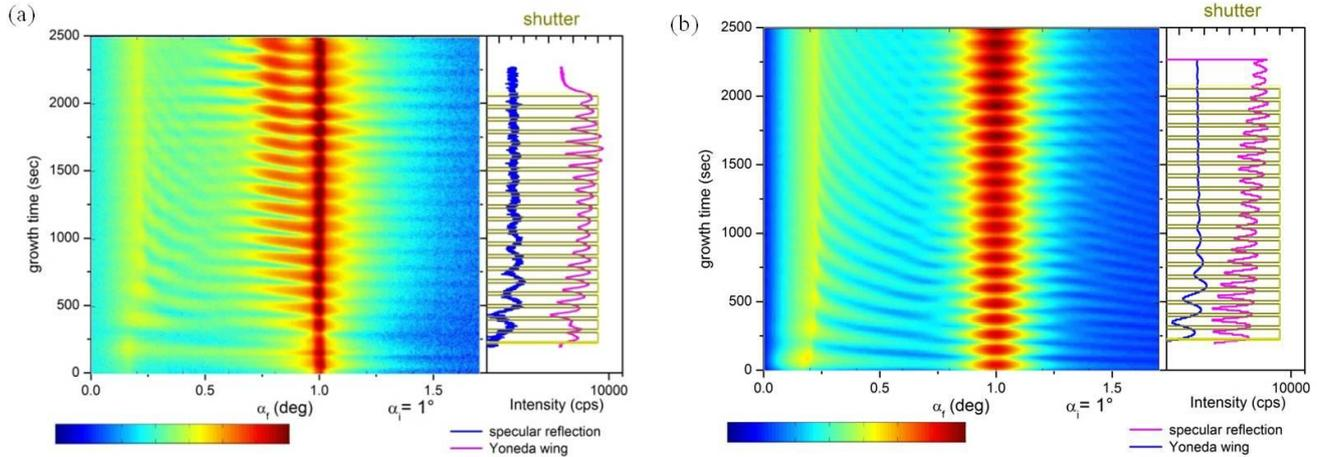
Figure 1. Experimentally measured time-scans of XRR on the growing films (multilayer left, a continuous Ge+Al<sub>2</sub>O<sub>3</sub> layer right) measured for incidence angle  $\alpha_i=1$  deg.
