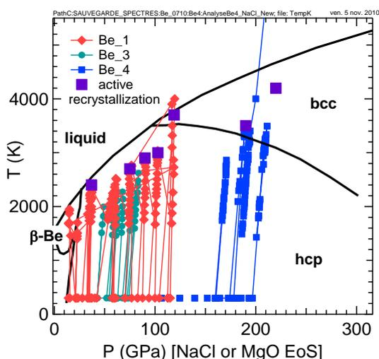
**Figure 1:** P-T paths followed in our diamond anvil cell experiments. The phase diagram proposed in [2] is represented in black. Temperature has been measured by pyrometry, pressure using NaCl or MgO pressure standards. The purple squares correspond to the conditions at which active recrystallization has been observed. They can be considered as a lower bound for the experimental melting curve.
