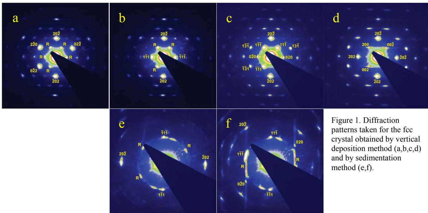
Figure 1. Diffraction patterns taken for the fcc crystal obtained by vertical deposition method (a,b,c,d) and by sedimentation method (e,f).
