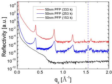
**<u>Figure 1</u>**: Out-of-plane post growth scan of 50nm PFP films at three substrate temperatures.
