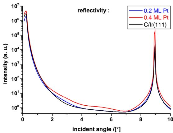
Fig. 2: specular rod for different Pt coverages – the distance of the oscillations reveals the layer thickness.
