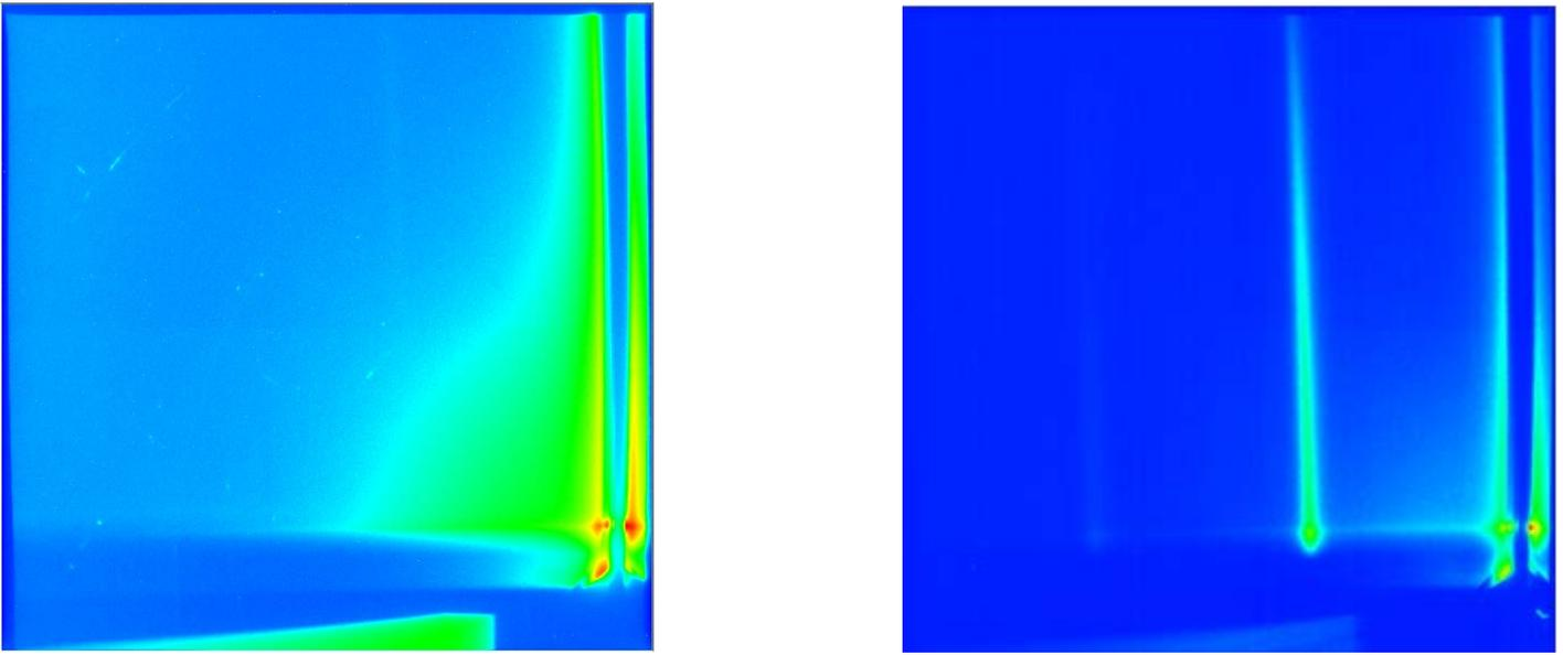
Fig. 1: (left) GISAXS image of graphene on Ir(111) – 35 sec. counting time. The weak first order graphene superstructure peak is observable. (right) GISAXS image of 0.4 ML Pt on graphene/Ir(111) – 1 sec. counting time. Due to the scattering contribution of Pt two orders of superstructure peaks are observable.
