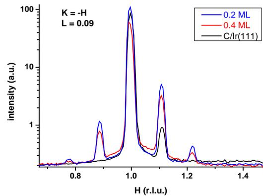
Fig. 3: in-plane linescans disclose superstructure periodicity particle strain and shape (envelop function).
