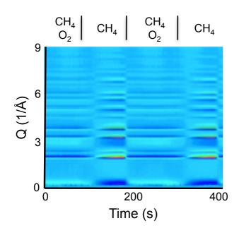
Figure 1. Structural dynamics in the active and promoter phases of a Pt/ceria catalyst during transient methane oxidation at 400°C observed *in situ* with HXRD.
