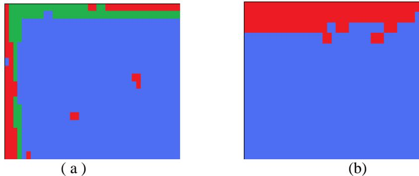
Figure 4: Corrosion in sensorglass after (a) 4h in a pH 4 solution and (b) 6h in a pH 7 solution (blue = original glass, green = corroded glass, red = resin)
