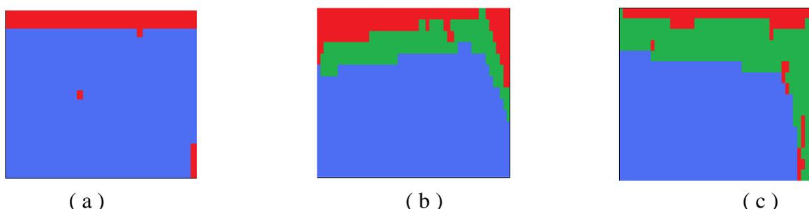
Figure 2: Cluster analysis map after (a) 0h, (b) 3h and (c) 6h in 1M HCl solution (blue = original glass, green = corroded glass, red = resin)
