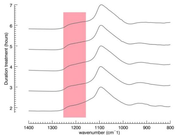
Figure 5: spectrum of leached layer as a function of treatment time
