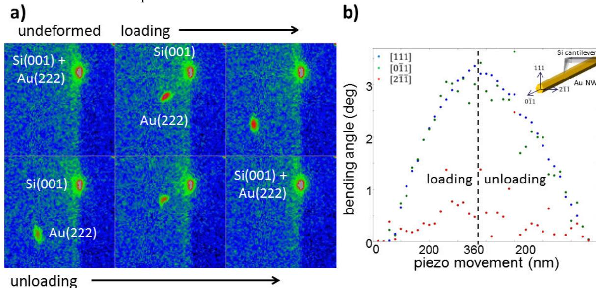
Fig. 3: a) *In situ*  $\mu$ Laue diffraction patterns recorded during the bending of a Au nanowire and b) bending angle computed from the position of the Laue spots.
