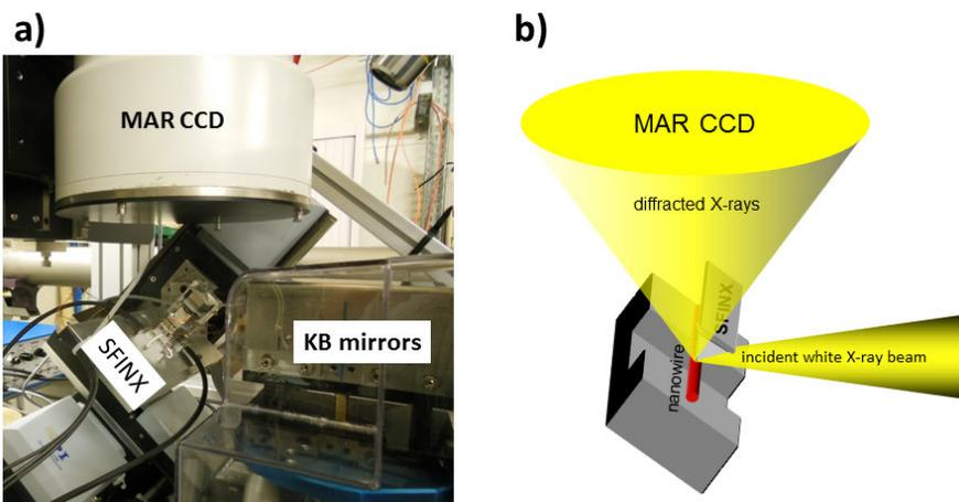
**Fig. 1:** a) Photograph and b) schematic of the experimental setup at the BM32 beamline including SFINX.
