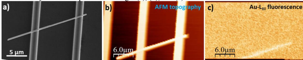
Fig. 2: a) Scanning electron microscopy image, b) *in situ* AFM image, and c) *in situ* fluorescence map of a single Au nanowires crossing a Si micro-trench.
